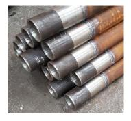
The cost of sponsoring these tubes includes the machining of the bottle ends, welding, X-raying, tapping of the holes in the firebox tube plate and the actual fitting process which involves screwing them into the firebox tube plate, expanding both ends and beading in the firebox
